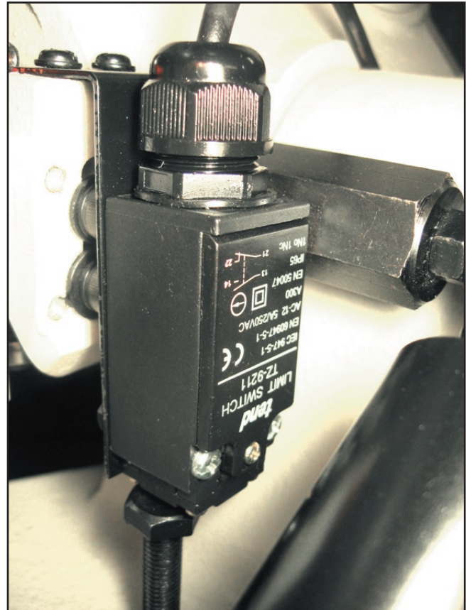
Figure 72. G0614 blade stop limit switch.
